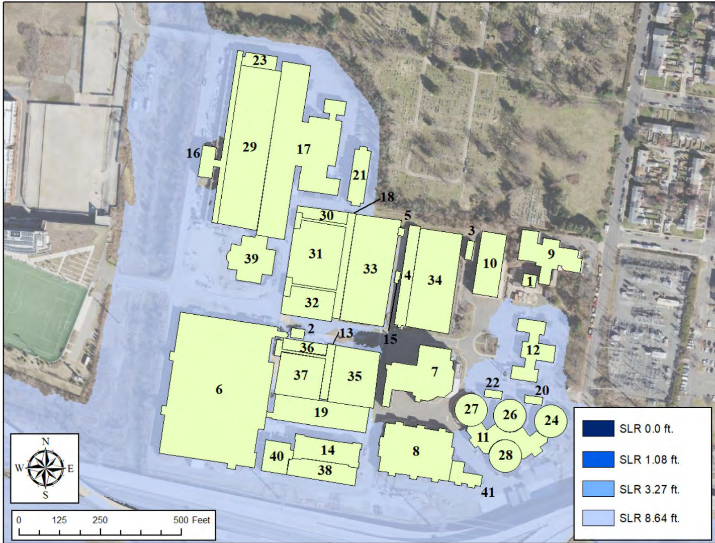
Figure 6.3: AlexRenew WWTP, 100-year coastal storm. Inundation of AlexRenew WWTP components and structures given existing sea level and three sea level scenarios (1.08 ft., 3.27 ft., and 8.64 ft.).
